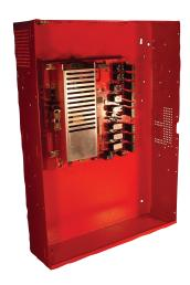
Use the FPP-RNAC-8A-4C power supply to add four additional notification appliance circuits to a fire alarm control panel (when connected via the option bus), or as a NAC power supply for fire-protective signaling systems (when connected directly to the NAC output). The additional notification appliance circuits can be NFPA 72, Class B (Style Y) or Class A (Style Z).
