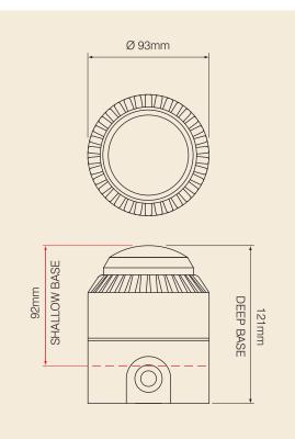
The Flashni is an audible and visual device which requires one single installation point. This greatly reduces installation and costs and is much less obtrusive than two separate devices. Versions are available with the sounder and beacon linked, or with separate terminals for independent operation.
