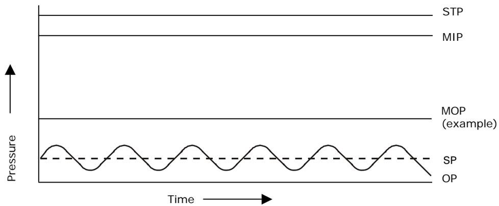
STP = strength test pressure
