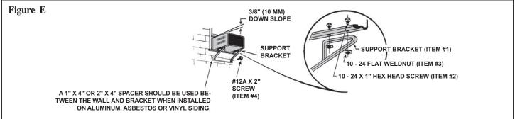
**STEP 3** OUTSIDE SUPPORT MOUNTING: Assemble the support brackets (Item #1) to the bottom rails of the cabinet with four (4) 10-24 1" long screws (Item #2) and four (4) 10–24 flat nuts (Item #3). Adjust the support brackets to bring the bottom pads in contact with the wall surface. (See Figure E.)
