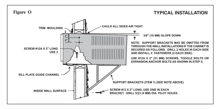
NOTE: ALTERNATE FASTENERS WHICH MAY BE USED FOR SECURING THE SILL PLATE IN THE WALL, AND THE SUPPORT BRACKETS TO THE OUTSIDE WALL ARE NOT FURNISHED, BUT ARE AVAILABLE AT A LOCAL HARDWARE STORE.
