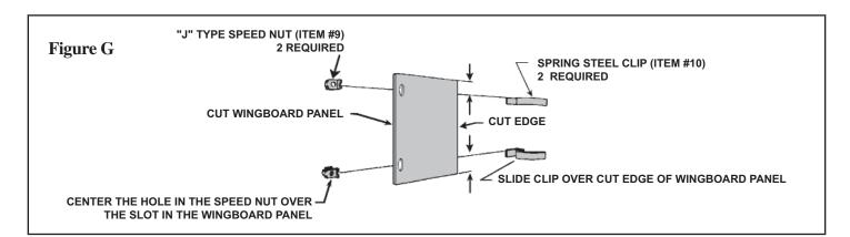
STEP 5 ASSEMBLE CLIPS TO WINGBOARD PANELS: Assemble "J" type speed nuts (Item #9) and spring steel clips (Item #10) to the edges of the cut wingboard panels (See Figure G).
